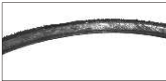
Shining surface due to high slippage
